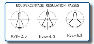
A total flow ball valve has been originally designed to have a high flow rate coefficient. To obtain a stabile and precise regulation that KV coefficient has to be reduced. It is possible then to get a linear modulation of irradiate heat as a function of shutter position.
